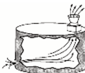
Effective Ventilation – Diagonal airflow
